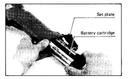
• Do not use force when inserting the battery cartridge. If the cartridge does not slide in easily, it is not being inserted correctly.
